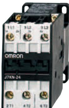
This modular system consists of main contactors and additional contact blocks. The basic units can be combined with auxiliary contacts. AC and DC versions, integrated mechanical interlock, are available as well as 3-main-pole and 4-main-pole versions.
