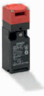
The D4NS line-up includes three-contact models with 2NC/1NC and 3NC contact forms in addition to the previous contact forms, 1NC/1NO and 2NC. Models with M12 connectors and conduit opening, such as M20, are also available.
