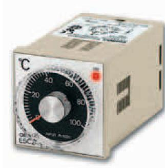
Omron's basic ON/OFF or PD controller features an analogue setting dial. This compact, low-cost controller has a setting accuracy of 2% of full scale. It incorporates a plug-in socket allowing for DIN-rail or flush mounting.
