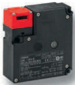
The D4NL guard-lock safety door switches are available with four or five built-in contacts. When locked, they have a key holding force of up to 1300N. Mechanical lock/solenoid release types and vice versa set up the complete range in combination with various conduit types, e.g. M20.
