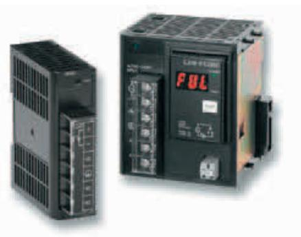
CJ1 systems can operate on 24 V DC power supply, or on 100 - 240 V AC mains. For small-scale systems with mainly digital I/O a low-cost small-capacity power supply can be used. For systems with many analog I/Os and control/communication units, it may be necessary to use a larger power supply Unit.
