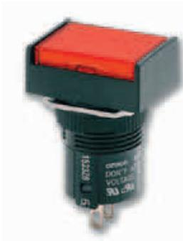
These subassembled pushbutton switches have a modular construction: pushbutton + case + lamp (if applicable) + switch. A16 is a nut-mounted pushbutton switch with a short mounting depth of less than 28.5mm below panel.
