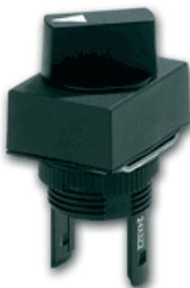
A165S/W nut-mounted, knob-type selector switches have a modular construction and a short mounting depth of less than 28.5mm below the panel. They come in a wide range of switching capacities, from standard load to micro load.
