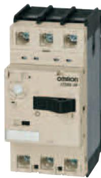
The J7MN motor starters protect motors against thermal overload and short circuit. The Motor protection circuit breakers can be equipped with additional auxiliary contacts, front or side mounted. Other options are circuit trip alarm units, undervoltage and shunt release units. To make wiring easy we provide as well busbar system.
