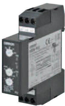
The K8DS-PU is the simplified 3-phase monitoring relay, 3-wire circuits within one unit. It can monitor undervoltages, phase sequence and phase loss.
