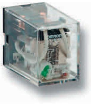
The LY series is equipped with arc barrier and built-in diode. LY comes in single-, double-, three- and four-pole models. The available mounting types are DIN-rail by socket, PCB & flange mounting.
