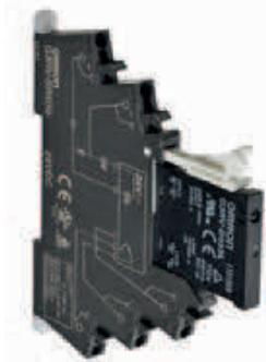
As well as being slim and thus saving panel space, G3RV relays are very strong, have a large contact area and non-bendable pins. Connection to a PLC is easy and achieved faultlessly in a few seconds via click connectors. In addition, power switching in G3RV relays with DC outputs is managed by a MOSFET in the output, which has ideal heat dissipation characteristics.
