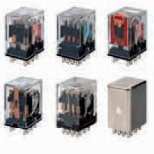
MY family has as standard feature on all models\* like: transparent cover, mechanical indicator to easily check the contacts status and the LED not only to indicate the correct operation of the relay, but also to immediate identify the coil voltage type: red LED for AC coil and green LED for DC coil
