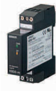
The K8DS-PH1 is a monitoring relay designed at only 17.5 mm wide with simplified functions for 3-phase 3 wire supplies. It simultaneously monitors phase sequence and phase loss during start up as well as phase loss during operation. The output relay releases when alarm conditions are detected, and the warning status can easily be monitored using the LED indicator.
