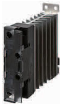
Single-phase SSR for low heat generation enables carrying 25 A (G3PJ-25B(-PU)) even for close mounting of three SSRs to contribute to downsizing of control panels. Models available with push-in plus input terminals.
