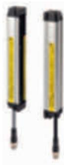
The F3SJ-B-family is a type 4 safety light curtain with an optical resolution of 25 mm. An operation range of up to 7 m and a protective height up to 2,065 mm are provided with no dead zone.
