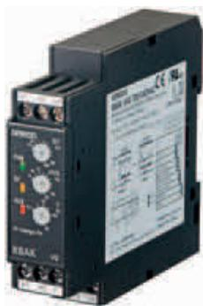
These single-phase voltage relays are for monitoring over- and undervoltages. Manual resetting and automatic resetting are supported by one relay. Relay warning status can easily be monitored using the LED indicator.
