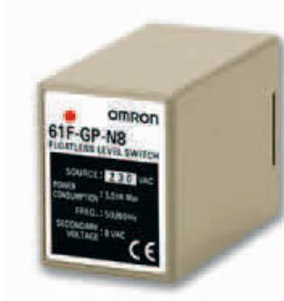
The 61F-GP-N8 can be used for single- or two-point level control of conductive materials, both liquids and solids. These products are equipped with a red LED operation indicator.
