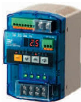
The S8M turns your machine directly into UL Class 2 compliant, maximum tripping current is 3,8A per channel (adjustable). This unit controls up to 4 circuits. On top of this you will get startup / shutdown –sequence control, display and alarm functions, like voltage, output current, runtime, and over temperature and external reset. These functions can be set by using the front buttons or with the free support tool software. These settings can be protected.
