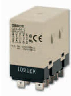
With a rated load current of 25A due to the miniature hinge for maximum switching power, the G7J can switch both motor loads as well as resistive and inductive loads. G7J has no contact chattering for momentary voltage drops up to 50% of its rated voltage.
