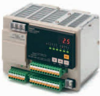
The S8AS series are smart power supplies with digital circuit protectors in a single package. The output is divided to 6 or 8 channels and provides adjustable tripping current range for each channel at 0.1 A increments. It can save installation space in panel with less-wiring by the integration of the circuit protector functions.
