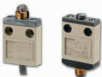
The 16 mm flat and compact size make the D4C range of limit switches very popular for all standard applications but especially where mounting space is limited or protruding housings may interfere with machine operation. The triple sealed construction, the rugged metal housing and the precisely manufactured movable parts ensure long operational life in standard or oily environments (special models).
