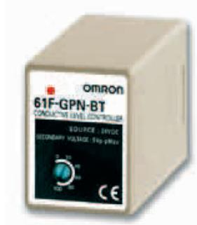
This controller is for single- or two-point level control. 24VDC supply allows for usage in locations without AC power supply. Relay contact chattering usually caused by waves has been eliminated by using open collector output, reducing contact wear.
