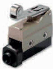
The compact housing size and the terminal block with side facing cable exit allow the mounting where space is crucial and self-wiring connection is preferred. The rugged and tight housing construction provides high protection while the low-force actuators make the ZC limit switch ideal for switching smaller or lighter objects.
