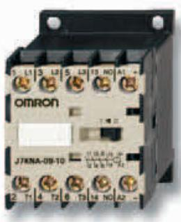
This modular system consists of main contactors and additional contact blocks. The basic units can be combined with auxiliary contacts (top mounting). Reversed versions, including integrated mechanical interlock, are available as well as 3-main-pole and 4-main-pole versions.
