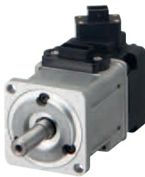
Accurax G5 servomotors include IP67 protection and connectors on the motor body. Use of 10 pole motors and 20 bit encoder results in 40% reduction in motor cogging. The servomotors are 25% lighter and 15% smaller due to patented new stator design PAC-Clamp, 40% iron loss reduction and 15% smaller encoder.
